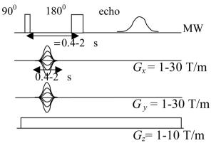
Fig. 1. Typical pulse imaging sequence employed in ESRM. Phase gradients shaped as "half sinus" wave are used for spatially encoding the *x* and *y*-axes of the sample, while a constant gradient is used along the *z*-axis. Typical peak values of the pulsed  $(G_x, G_y)$  and the constant  $(G_z)$  field gradients are shown. (See also refs 16,19 for more details.)
