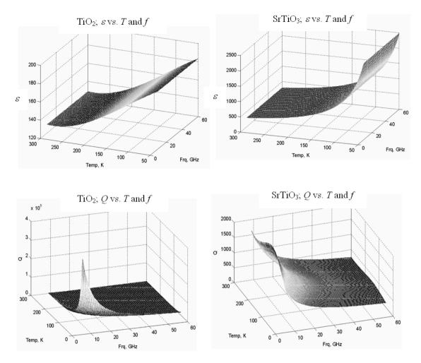
Fig. 6. The calculated permittivity ( $\epsilon$ ) and Q of SrTiO<sub>3</sub> and TiO<sub>2</sub> single crystals vs. temperature and frequency.
