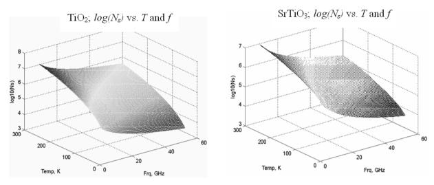
Fig. 7. The calculated minimum number of detectable electron spins by pulsed ESRM after 60 min of of acquisition (Ns), employing resonators based on SrTiO<sub>3</sub> and TiO<sub>2</sub> single crystals vs. temperature and frequency.
