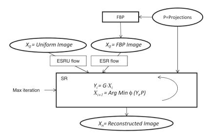
**Fig. 1.** Flowchart schematically showing the different processing approaches using EsrSr and EsrSrU. The raw projections P are used to create the FBP image and inside the Statistical Reconstruction algorithm. The EsrSrU starts from a uniform image  $X_0$  while the EsrSr starts from the FBP image. The stopping criterion of the algorithm is a specified maximum number of iterations n, and  $X_0$  is the final reconstructed image.
