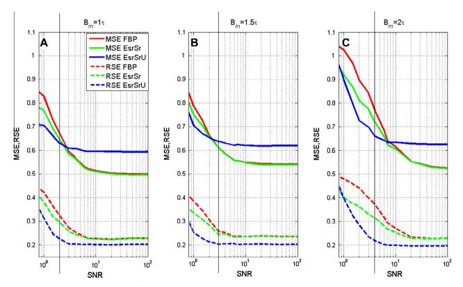
**Fig. 5.** Spatial–spatial – MSE and RSE vs. SNR for different modulation intensities. (A) Modulation amplitude  $B_m$  is equal to  $\tau$ , (B)  $B_m$  = 1.5 $\tau$  and (C)  $B_m$  = 2 $\tau$ . The SNR is plotted in a logarithmic scale for values from 0.8 to 100 while the number of projections is held constant in this simulation (see Section 5.3.1). The three doted vertical lines indicate the working points presented in Figs. 2–4, respectively.
