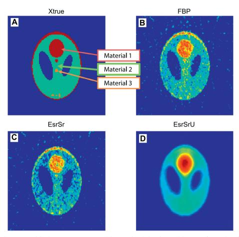
**Fig. 6.** Spectral-2D spatial phantom- central slice image;  $B_m = 2\tau_{\min}$ , SNR = 10. (A) Xtrue – the noiseless phantom; (B) FBP–FBP after negative values cancelation; (C) EsrSr – with postreconstruction cancellation of negative values, the initial image is the FBP; (D) EsrSrU – with postreconstruction cancellation of negative values, the initial image is uniform.
