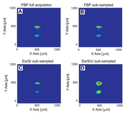
Fig. 12. Spatially-resolved ESR spectra: spatial–spatial slices for LiPc spectrum,  $B_m = \tau_{\min}$ , While full acquisition refers to 4096 projections, subsampled data refers to 1024 projections. (A) FBP – full acquisition, (B) FBP – subsampled (C) EsrSr – subsampled, (D) EsrSrU – subsampled.
