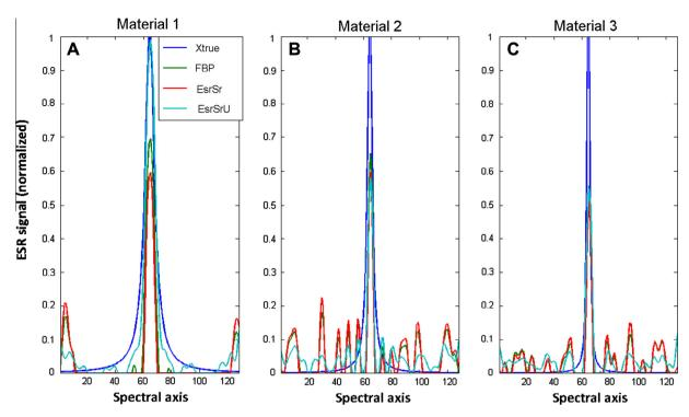
**Fig. 9.** Spectral-2D spatial phantom profiles along the spectral dimension (the 2-Gauss span is divided to 128 points);  $B_m = 3\tau_{min}$ . SNR = 15. (A) Material 1 at the central position in red in Fig. 6, (B) Material 2 at the central position in green in Fig. 6, finally (C) Material 3 at the central position in orange in Fig. 6.
