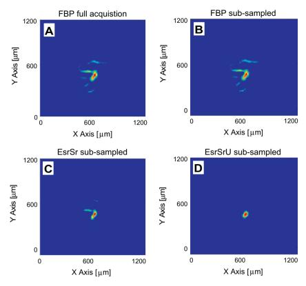
Fig. 13. As in Fig. 12, spatial-spatial slices for LiNc-BuO spectrum, (A) FBP Full acquisition, (B) FBP – subsampled, (C)EsrSr – subsampled, and finally (D) EsrSrU – subsampled.
