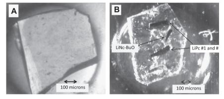
Fig. 10. (A) Optical image of the LiNc–BuO sample used in our 2D spatial imaging experiments. (B) Optical image of a sample containing both LiPc and LiNc–BuO crystals employed in our spectral-2D spatial imaging experiments.
