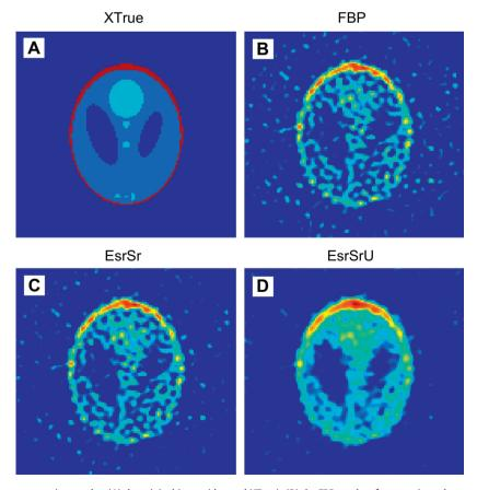
**Fig. 2.** Spatial–spatial phantom reconstruction results: (A) the original image (denoted XTrue); (B) the FBP results after negative value cancelation; (C) the EsrSr algorithm-reconstructed image using nonnegativity constraints and the FBP image as the initial image; (D) same as (C) but using a uniform image as initial image (denoted EsrSrU). In all images, the projection SNR = 2 and the modulation amplitude,  $B_m$ , is equal to the FWHM line-width of the given ESR spectrum ( $B_m = \tau$ ).
